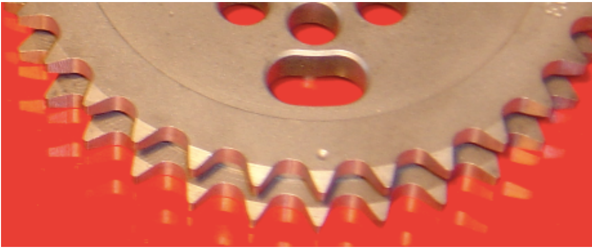
Figure 5; Note timing Dot on the original cam sprockets
