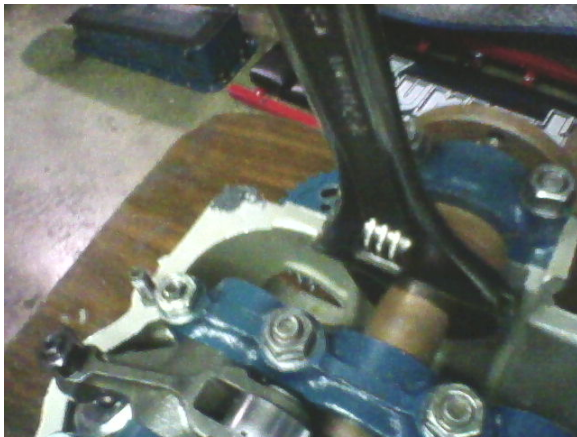
Figure 3 Rotate cams with an open end via one of the two flats
