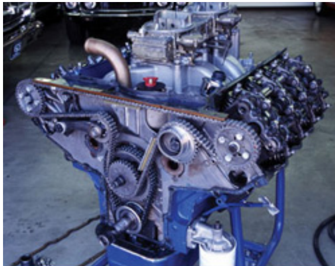
Figure 1; Internet picture of original chain drives
